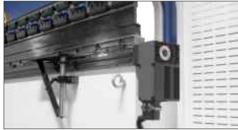
Deflection compensation structure
