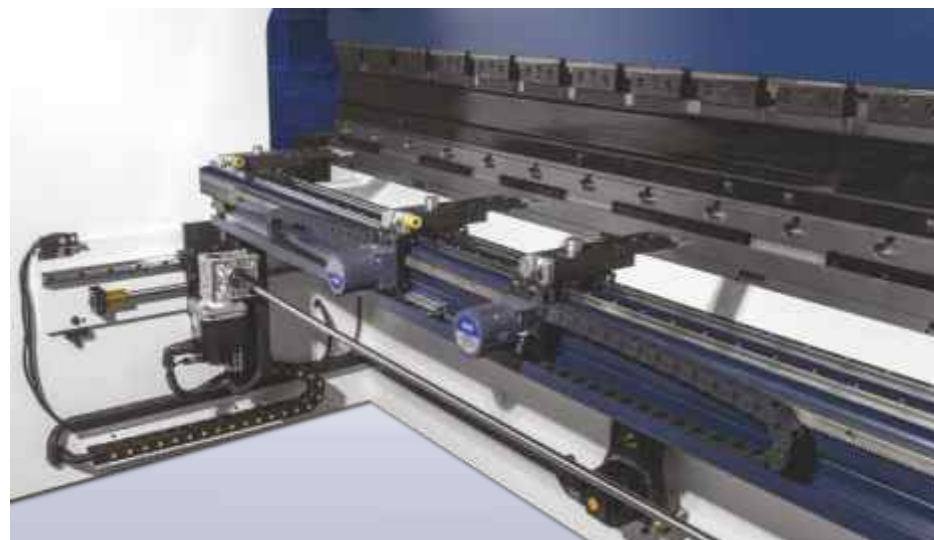
6+1 axis CNC backgauge (Y1+Y2+X+R+Z1+Z2)+V
